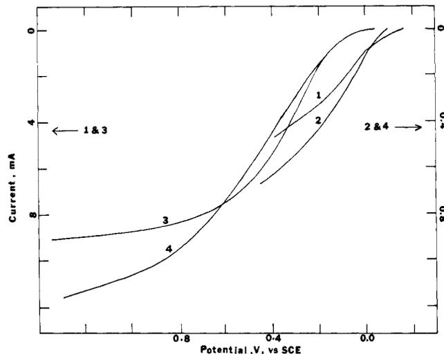
**Figure 3.** Current-potential curve for illuminated polycrystalline  $\text{TiO}_2$  in the presence and absence of *p*-aminophenol (PAP): (1) 30 mM PAP in 0.2 M  $\text{H}_2\text{SO}_4$  at full lamp intensity; (2) 30 mM PAP in 0.2 M  $\text{H}_2\text{SO}_4$  with neutral density filters; (3) 0.2 M  $\text{H}_2\text{SO}_4$  at full lamp intensity; (4) 0.2 M  $\text{H}_2\text{SO}_4$  with same filters as (2).
