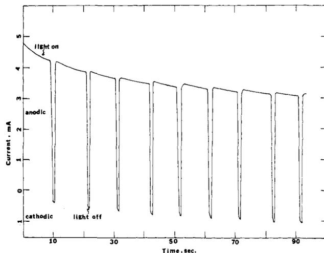
Figure 8. Current-time behavior of 1 M NaBr at TiO<sub>2</sub> on platinum with fuel cell cathode (no external power supply) with and without light from 450 W Xenon lamp. Current measured through 1 Ω resistor connected between anode and cathode.
