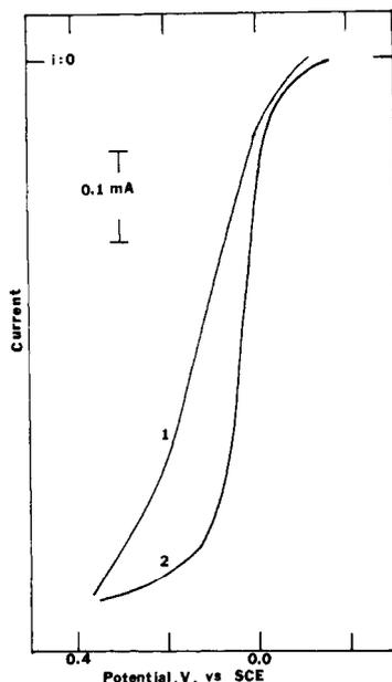
**Figure 4.** Current-potential curve for illuminated single crystal  $\text{TiO}_2$  in the presence and absence of PAP. Output of 450 W Xenon lamp attenuated with neutral density filters: (1) absence of PAP, 0.2 M  $\text{H}_2\text{SO}_4$ ; (2) presence of 30 mM PAP in 0.2 M  $\text{H}_2\text{SO}_4$ .
