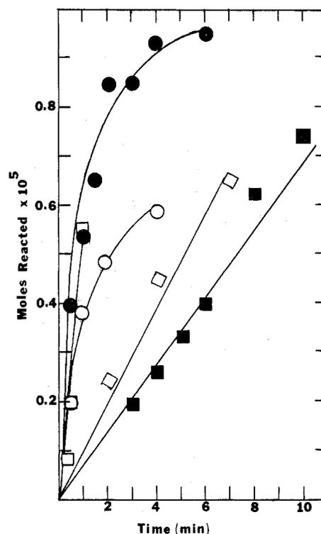
Figure 3. Number of mol of  $\text{SO}_3^{2-}$  that reacted in 10 mL of 1 mM  $\text{Na}_2\text{SO}_3$  (also 10 mM acetic acid) following illumination with 450-W xenon lamp while bubbling  $\text{O}_2$ . Solution also contained (●) 0.1 g of  $\text{Fe}_2\text{O}_3$  powder, (□) 0.1 g of ZnO powder, (○) 0.1 g of CdS powder prepared in this lab, (◇) 0.1 g of CdS powder, commercial, (■) 0.1 g of anatase  $\text{TiO}_2$  powder.
