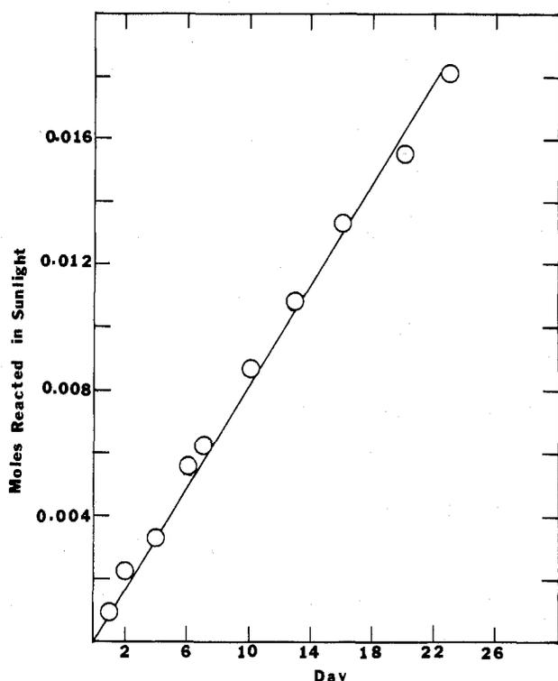
**Figure 2.** Number of mol of  $\text{CN}^-$  that reacted in 750 mL of a 30 mM KCN solution (0.1 M KOH) containing 7.5 g of anatase  $\text{TiO}_2$  illuminated with unfocused sunlight. The solution was unstirred.
