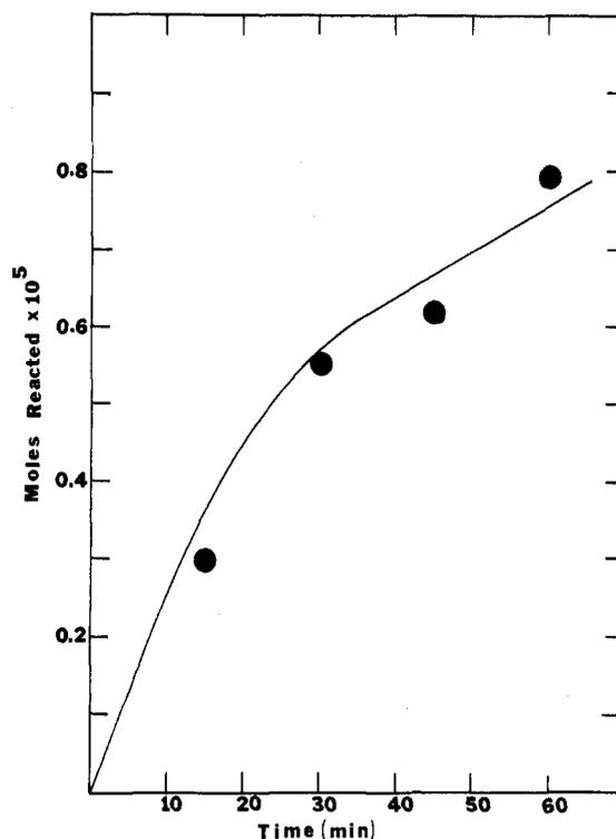
Figure 1. Number of mol of  $\text{CN}^-$  that reacted following irradiation with 450-W xenon lamp while bubbling  $\text{O}_2$ . Solution initially 1 mM  $\text{CN}^-$ . 0.1 M KOH electrolyte containing 0.1 g of anatase  $\text{TiO}_2$ . Solution volume 10 mL.
