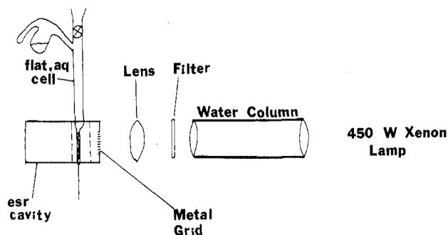
Figure 1. Experimental apparatus for the detection of radical intermediates during the illumination of TiO<sub>2</sub> powder samples.
