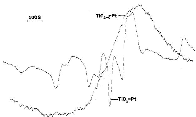
**Figure 6.** Experimental spectra of reduced and unreduced platinized TiO<sub>2</sub> (anatase) powders in aqueous media.
