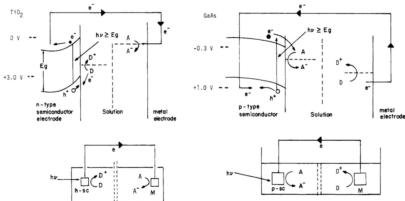
**Figure 3.** Schematic representation of (A) n-type semiconductor photoelectrochemical cells with typical values for the band-edge locations for n-TiO<sub>2</sub> at pH 0 (V vs. NHE). (B) p-type semiconductor cell with band-edge locations for p-GaAs at pH 0.
