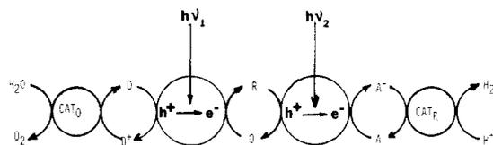
**Figure 6.** Schematic diagram of a solar energy utilization system employing two light absorbers and requiring two photons (at energies  $h\nu_1$  and  $h\nu_2$ ) to drive one electron through the system. The system is similar to that in Figure 1, except that an intermediate redox couple, O/R, connects the two light-absorbing systems.
