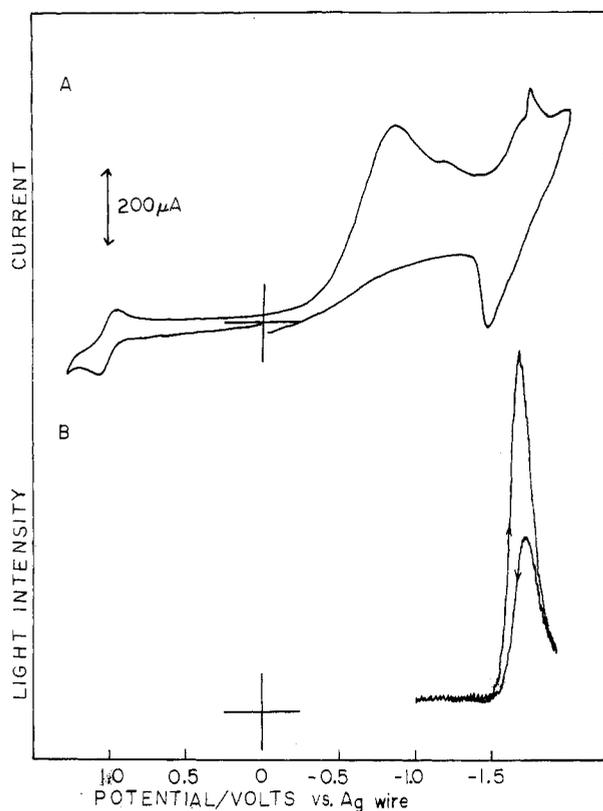
Figure 3. (A) Cyclic voltammogram for 2 mM  $\text{Ru}(\text{bpy})_3^{2+}$  in a (1:1)  $\text{CH}_3\text{CN}/\text{H}_2\text{O}$  mixture, 0.1 M  $\text{TBABF}_4$  in the presence of 10 mM  $\text{Na}_2\text{S}_2\text{O}_8$ , at a GC electrode, at a sweep rate of  $100 \text{ mV s}^{-1}$ ; (B) light intensity vs. potential profile for the solution in (A).
