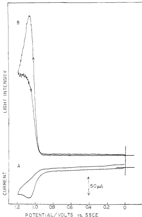
Figure 1. (A) Cyclic voltammogram for 1 mM  $\text{Ru}(\text{bpy})_3^{2+}$  in pH 5 phosphate buffer in the presence of 30 mM  $\text{Na}_2\text{C}_2\text{O}_4$ , at GC electrode, at a sweep rate of  $50 \text{ mV s}^{-1}$ ; (B) light intensity vs. potential profile for the solution in (A).
