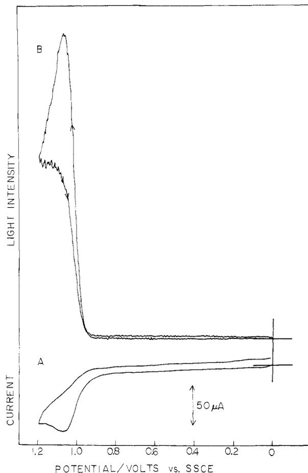
Figure 1. (A) Cyclic voltammogram for 1 mM  $\text{Ru}(\text{bpy})_3^{2+}$  in pH 5 phosphate buffer in the presence of 30 mM  $\text{Na}_2\text{C}_2\text{O}_4$ , at GC electrode, at a sweep rate of  $50 \text{ mV s}^{-1}$ ; (B) light intensity vs. potential profile for the solution in (A).
