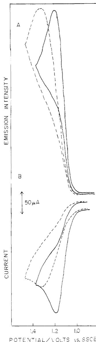
**Figure 5.** (A) ECL light intensity as a function of potential for 1 mM  $\text{Ru}(\text{bpy})_3^{2+}$  in the oxalate system in the absence (—) and in the presence (---) of liver tissue extract and ascites fluid; (B) single sweep voltammograms for the solution in (A) at a GC electrode at a sweep rate of  $50 \text{ mV s}^{-1}$ . Oxalate concentration is 30 mM.
