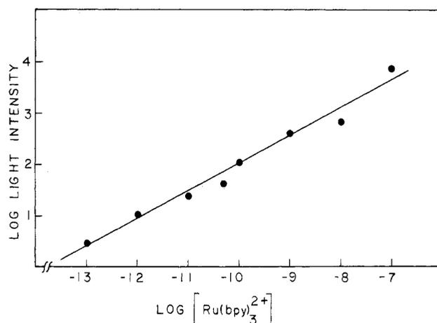
Figure 4. log-log plot of the observed light intensity vs.  $\text{Ru}(\text{bpy})_3^{2+}$  concentration.
