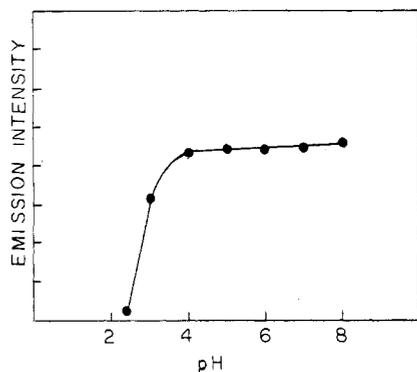
Figure 2. ECL light intensity dependence of a 0.6 mM  $\text{Ru}(\text{bpy})_3^{2+}$  solution on pH, in phosphate buffer ( $\mu = 0.2$ ), in the presence of 27 mM  $\text{Na}_2\text{C}_2\text{O}_4$ .
