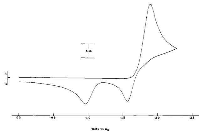
**Figure 1.** Cyclic voltammogram of 3.71 mM  $[\text{Rh}(\mu\text{-}t\text{-Bu}_2\text{P})(\text{CO})_2]_2$  in THF/0.5 M (TBA)BF<sub>4</sub> scanned between 0.00 and -2.25 V. Scan rate 200 mV s<sup>-1</sup>.
