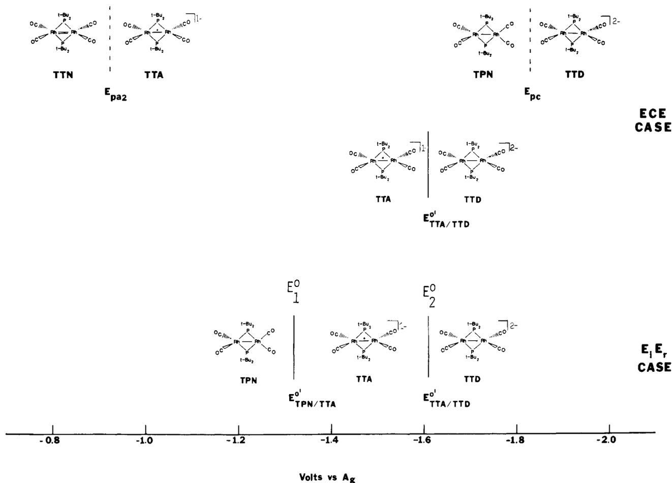
Figure 6. Summary of peak potentials and  $E^\circ$  values for the ECE/EEC-Disp and  $E_1E_2$ -Disp mechanisms. Peak potentials are those observed at 200  $\text{mV s}^{-1}$ .
