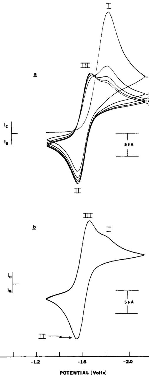
**Figure 2.** Cyclic voltammograms of 3.71 mM  $[\text{Rh}(\mu\text{-}t\text{-Bu}_2\text{P})(\text{CO})_2]_2$  in THF/0.5 M (TBA)BF<sub>4</sub> scanned between -1.29 and -2.15 V. Scan rate 200 mV s<sup>-1</sup>. (a) First five scans; (b) steady state observed after ca. 10 scans.
