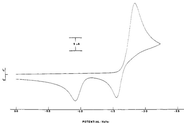
**Figure 4.** Simulated cyclic voltammograms for an ECE/EEC-Disp mechanism based on  $E_3^\circ = -1.24$  V,  $k_3^\circ = 1.6 \times 10^{-3}$  cm s $^{-1}$ ,  $\alpha_3 = 0.65$ , and the parameters listed for Figure 3. Scan rate and initial and switching potentials are the same as those listed for Figure 1.
