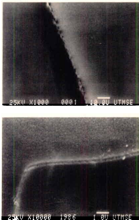
Figure 2: Scanning electron micrographs of n-GaAs electrochemically etched in an aqueous solution containing 5 mM NaOH and 1 mM EDTA. Irradiation with tungsten-halogen lamp. (a) Photoelectrochemical current, 3.2 \mu\text{A} ; Tip scan rate, 150 \text{ \AA/sec} ; Bias voltage, 4 V; Light and voltage pulsed, 5 sec on, 5 sec off. (b) Photoelectrochemical current, 0.7 \mu\text{A} ; Tip scan rate, 0.1 \mu\text{m/sec} ; Bias voltage 4 V; Light and voltage applied continuously and the tip was moved in an L-pattern.
