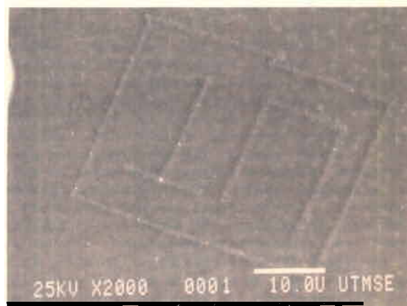
Fig. 2. Scanning electron micrograph of a pattern of silver lines deposited in a Nafion film. The bias voltage was 3V, with a tip scan rate of ca. 400 \text{ A s}^{-1} . Marker, 10 \mu\text{m} .
