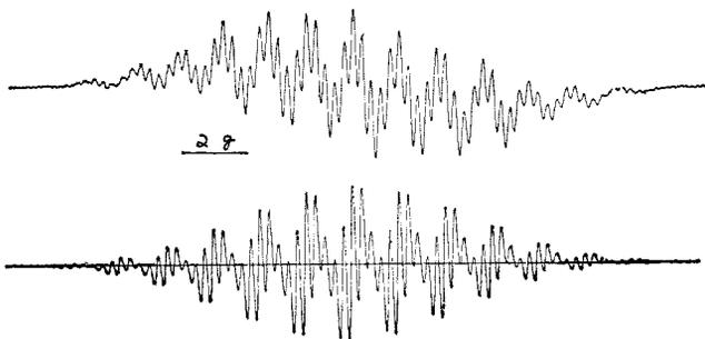
Figure 1. Top: derivative esr spectrum of DPA anion radical produced by electroreduction of  $10^{-3}$  M DPA solution containing 0.1 M tetra-*n*-butylammonium iodide in *N,N*-dimethylformamide. Spectrometer conditions: modulation amplitude, 0.1 gauss; power, 10 db; sweep time, 25 min. Bottom: calculated spectrum using constants in text.
