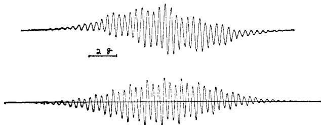
Figure 2. Top: derivative esr spectrum of DPA cation radical produced by treating a  $5 \times 10^{-3}$  M DPA solution in hexane with concentrated sulfuric acid. Spectrometer conditions: modulation amplitude, 0.07 gauss; power, 20 db; sweep time, 25 min. Bottom: calculated spectrum using constants in text.
