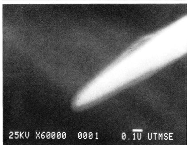
**Figure 2.** SEM micrographs of a Pt tip.
