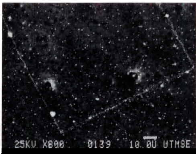
Fig. 11. SEM picture of gold deposited on a graphitic layer. Bias, -5V; other parameters are identical to the parameters in Fig. 6.
