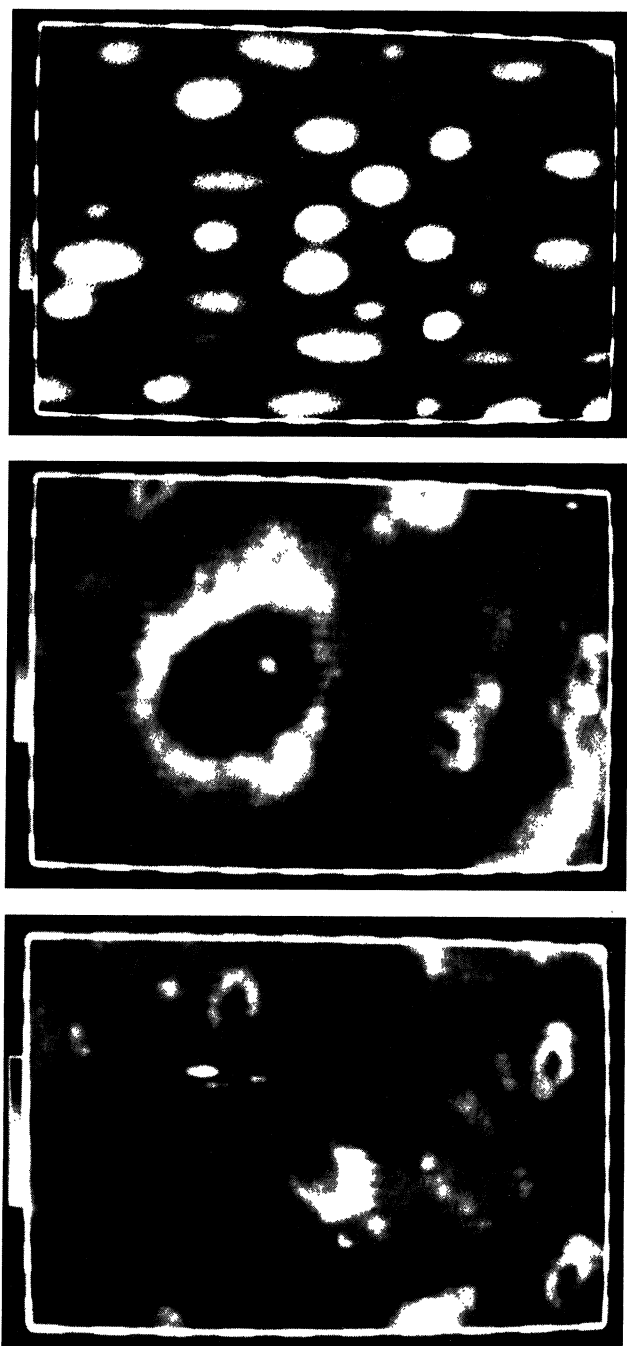
FIG. 2. Gray-scaled image of biological substrates in a \text{K}_4\text{Fe}(\text{CN})_6/\text{KCl} solution scanned with Pt UME (radius, 1 \mu\text{m} ). (Upper) Top surface of grass. (Middle and Lower) Bottom surface of L. sinensis leaf. Small openings are stomata.
