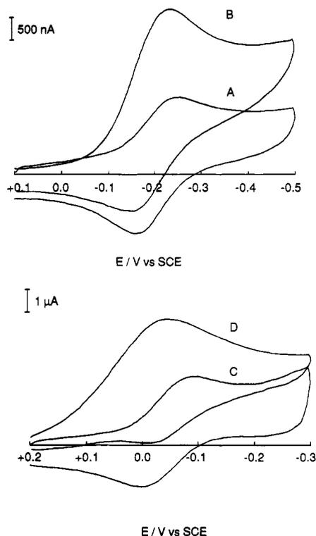
**Figure 2.** Cyclic voltammograms of (A, B) 0.50 mM Mn<sup>III</sup>-TMPyP and of (C, D) 0.78 mM Fe<sup>III</sup>-TMPyP, (A, C) in the absence and (B, D) in the presence of air (oxygen): sweep rate, 100 mV/s; supporting electrolyte, buffer 1.
