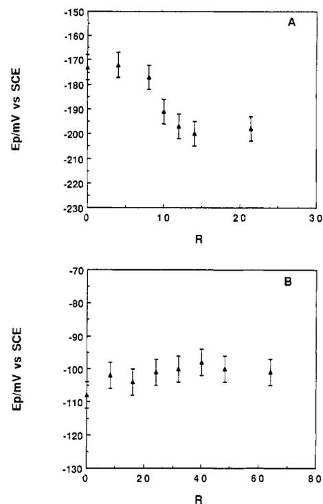
**Figure 4.** Effect of  $R$  ( $[NP]/[M^{III}TMPyP]$ ) on the DPV peak potential ( $E_p$ ) of (A) 0.1 mM Mn<sup>III</sup>-TMPyP (buffer 1) and (B) 0.1 mM Fe<sup>III</sup>-TMPyP (buffer 2).
