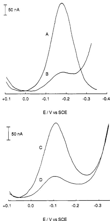
**Figure 3.** Differential pulse voltammograms of (A, B), 0.1 mM Mn<sup>III</sup>-TMPyP (buffer 1) and of (C, D) 0.1 mM Fe<sup>III</sup>-TMPyP (buffer 2), (A, C) in the absence of DNA and in the presence of sonicated CT DNA with (B) 0.8 mM NP, (D) 4.8 mM NP. Solutions were deoxygenated.
