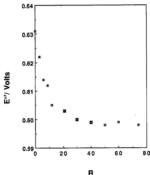
**Figure 2.** Effect of  $R$  ( $[\text{NP}]/[\text{Os}(\text{bpy})_3^{2+}]$ ) on  $E^{\circ'}$ :  $[\text{Os}(\text{bpy})_3^{2+}] = 0.1$  mM; supporting electrolyte, buffer 1; working electrode, glassy carbon (area, 0.088 cm<sup>2</sup>).
