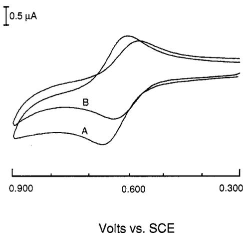
**Figure 1.** Cyclic voltammograms of 0.1 mM  $\text{Os}(\text{bpy})_3^{2+}$  (A) in the absence and (B) in the presence of 3.0 mM NP: sweep rate, 100 mV/s; supporting electrolyte, buffer 1; working electrode, glassy carbon (area, 0.088 cm<sup>2</sup>).
