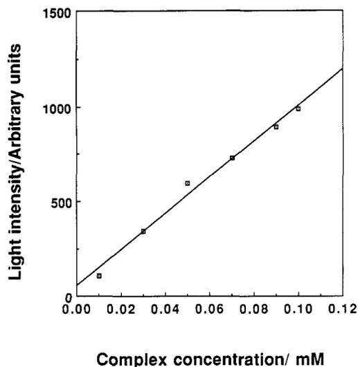
Figure 6. ECL dependence on  $\text{Os}(\text{bpy})_3^{2+}$  concentration: sweep rate, 438 mV/s; supporting electrolyte, buffer 2.
