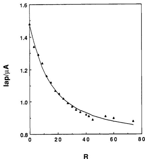
Figure 3. Cyclic voltammogram titration of 0.1 mM  $\text{Os}(\text{bpy})_3^{2+}$  with CT DNA: sweep rate, 100 mV/s; supporting electrolyte, buffer 1; working electrode, glassy carbon (area, 0.088 cm<sup>2</sup>).
