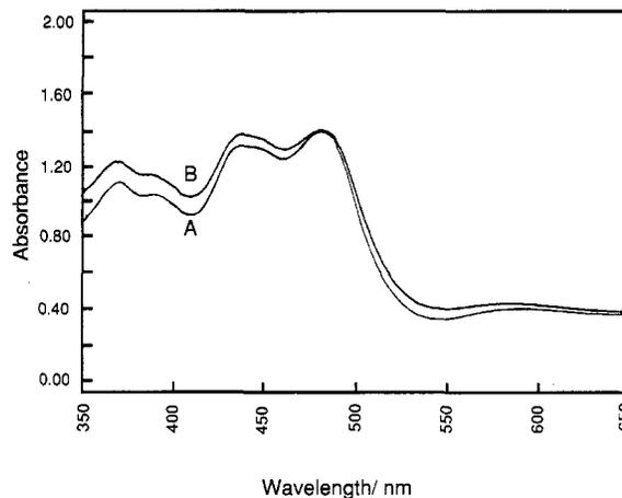
Figure 8. Absorbance spectra of 0.10 mM  $\text{Os}(\text{bpy})_3^{2+}$  (A) in the absence and (B) in the presence of 3.0 mM NP; buffer 2.
