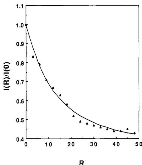
Figure 7. ECL titration of 0.1 mM  $\text{Os}(\text{bpy})_3^{2+}$  with CT DNA: sweep rate, 438 mV/s; supporting electrolyte, buffer 2.
