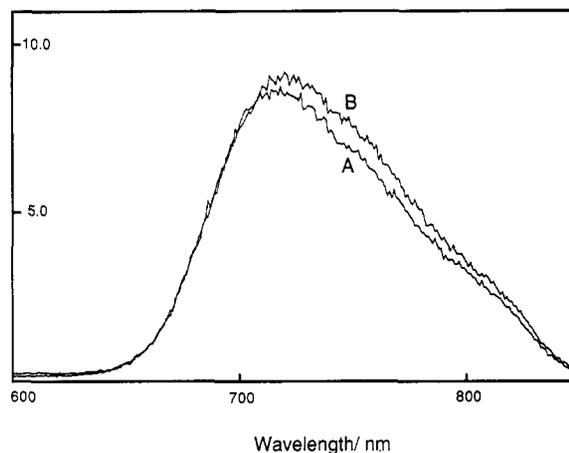
Figure 9. Photoluminescence spectra of 0.05 mM  $\text{Os}(\text{bpy})_3^{2+}$  (A) in the absence and (B) in the presence of 1.5 mM NP; buffer 2; excitation wavelength, 470 nm.
