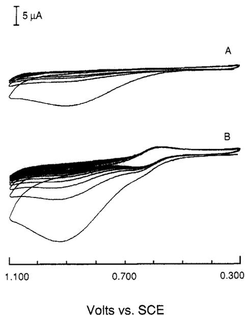
Figure 4. Cyclic voltammograms of 10.0 mM  $\text{C}_2\text{O}_4^{2-}$  (A) in the absence and (B) in the presence of 1.0 mM  $\text{Os}(\text{bpy})_3^{2+}$ : sweep rate, 100 mV/s; supporting electrolyte, buffer 2; working electrode, platinum disk (area, 0.023 cm<sup>2</sup>).
