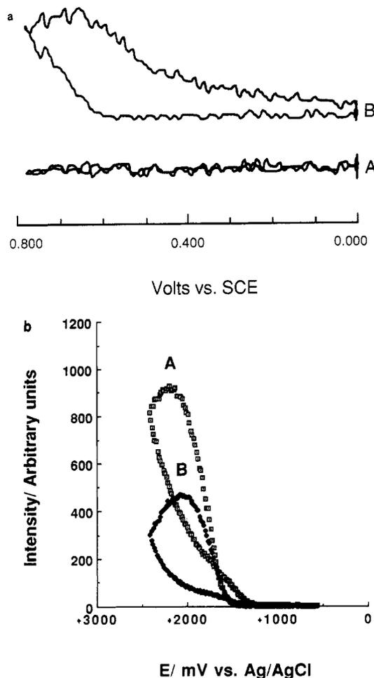
Figure 5. (a) ECL emission of a solution (A) without and (B) with 1.0 mM  $\text{Os}(\text{bpy})_3^{2+}$ : sweep rate 100 mV/s; supporting electrolyte, buffer 2; working electrode, platinum disk (area, 0.03 cm<sup>2</sup>). (b) ECL spectra of 0.1 mM  $\text{Os}(\text{bpy})_3^{2+}$  (A) in the absence and (B) in the presence of 2.4 mM NP: sweep rate, 438 mV/s; supporting electrolyte, buffer 2.
