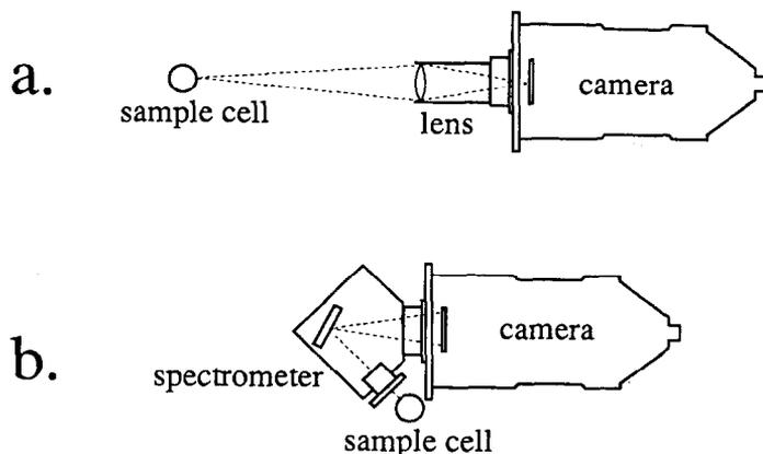
Fig. 1. (a) Schematic diagram of the experimental set-up for ECL imaging and light integration with the CCD camera; (b) set-up for ECL emission spectroscopy.
