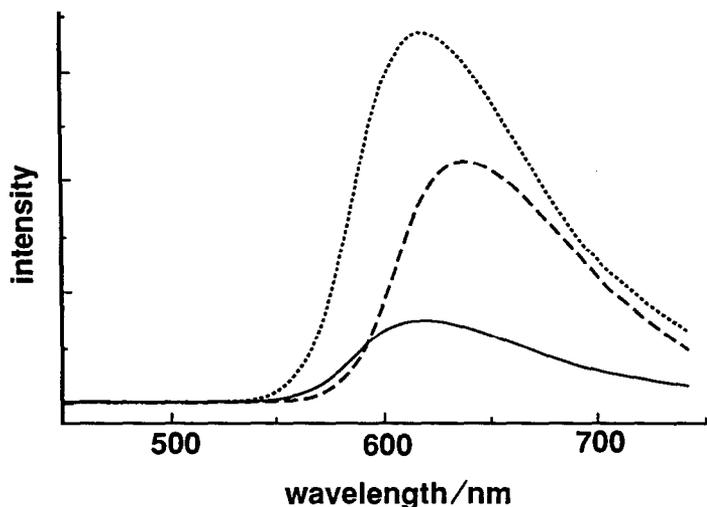
Fig. 3. ECL spectra of  $\text{Ru}(\text{bpy})_3^{2+}$  (—),  $\text{Ru}(\text{dp-bpy})_3^{2+}$  (---), and  $\text{Ru}(\text{dp-phen})_3^{2+}$  (·····). The solutions contained 0.1 M  $\text{TBABF}_4$  in MeCN. Intensities shown have been normalized to the concentrations of the complexes.
