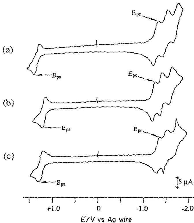
Fig. 2. Cyclic voltammograms of (a)  $\text{Ru}(\text{bpy})_3^{2+}$ , (b)  $\text{Ru}(\text{dp-bpy})_3^{2+}$ , (c)  $\text{Ru}(\text{dp-phen})_3^{2+}$ , all approximately 1.0 mM in 0.1 M  $\text{TBABF}_4$  in MeCN.
