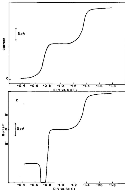
Fig. 1. Polarograms before and after reduction of a 1.32 mM APDO solution in DMF containing 0.1M TBAP at a mercury pool electrode: 1, before reduction; 2, after reduction at  $-1.0$  v vs. SCE.
