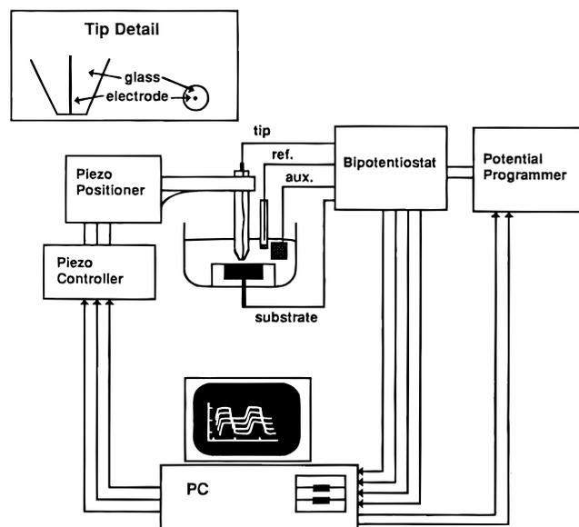
**Figure 1.** SECM apparatus. Reprinted with permission from Bard, A. J.; Denuault, G.; Lee, C.; Mandler, D.; Wipf, D. O. *Acc. Chem. Res.* **1990**, *23*, 357. Copyright 1990 American Chemical Society.
