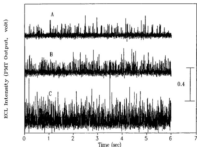
**Figure 9.** Histograms of the ECL intensity sampled at 1 kHz for three different gap separations between the tip and ITO substrate. Curves A, B, and C for *z* positions marked A and B in Figure 8A and for the tip far away from the substrate, respectively. Tip (*a* = 12.5 μm) and substrate biased at 2.1 and -0.3 V vs SSCE, respectively, during ECL generation in an acetonitrile solution containing 1 mM Ru(bpy)<sub>3</sub><sup>2+</sup>, 20 mM TPrA, and 0.2 M TBABF<sub>4</sub>.
