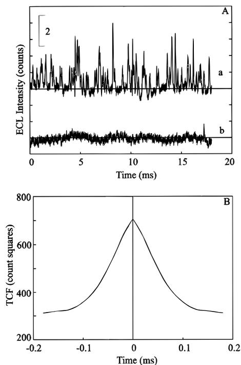
**Figure 11.** (A) Curve a: Histogram of the ECL intensity viewed at a sampling rate of 200 kHz. Tip far away from the ITO substrate. Conditions for ECL generation and the tip the same as those in Figure 9. Curve b: Background histogram. (B) Time correlation function (TCF) of curve a. ECL intensity experiments carried out with a Hamamatsu C1230 photon counter with a PMT R928P, which was cooled thermoelectrically to  $-15\text{ }^{\circ}\text{C}$ .
