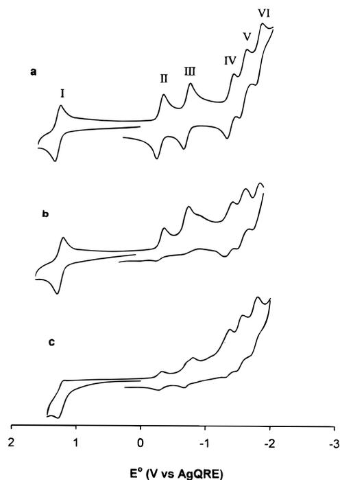
**Figure 2.** Cyclic voltammograms of a 0.7 mM solution of M2M in MeCN at a glassy carbon electrode (0.2 M TBAPF<sub>6</sub>; scan rate 200 mV/s) (a) before ECL, (b) with added oxygen, and (c) after extended ECL in the presence of air. Solutions in a and c are oxygen-free.
