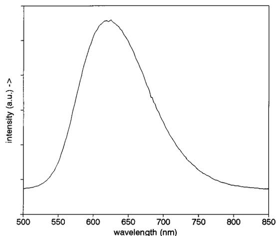
Figure 6. ECL emission spectrum of (bpy)<sub>2</sub>Ru(bphb)<sup>2+</sup> with (Bu<sub>4</sub>N)-S<sub>2</sub>O<sub>8</sub>. MeCN solutions were 1 mM in complex, 10 mM in (Bu<sub>4</sub>N)S<sub>2</sub>O<sub>8</sub>, and 0.1 M in Bu<sub>4</sub>NPF<sub>6</sub>. The S<sub>2</sub>O<sub>8</sub><sup>2-</sup> spectra were generated by pulsing of the electrode potential between 0 and -1.1 V. Holding time at each limit was 0.1 s.
