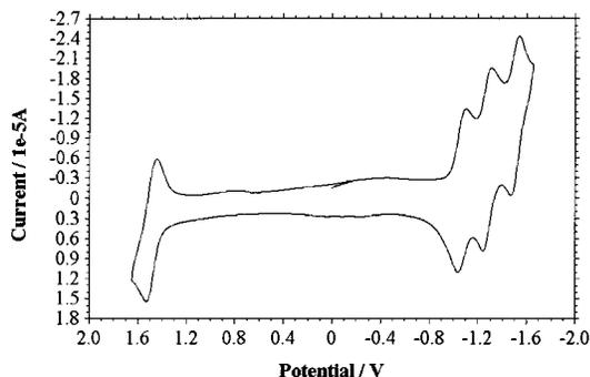
Figure 5. Cyclic voltammogram of (bpy)<sub>2</sub>Ru(bphb)(PF<sub>6</sub>)<sub>2</sub>. Same conditions as in Figure 2.
