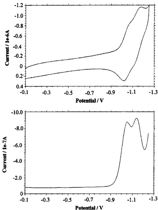
Figure 2. Reductive cyclic and square-wave voltammograms of 1 mM  $[(\text{bpy})_2\text{Ru}]_2(\text{bphb})(\text{PF}_6)_4$  in MeCN/0.1 M  $\text{Bu}_4\text{NPF}_6$ . Scan rate 100 mV/s.
