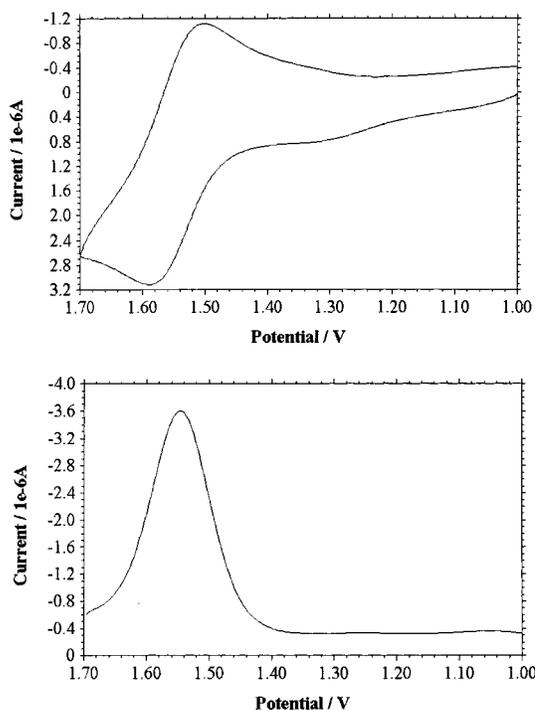
Figure 3. Oxidative cyclic and square-wave voltammograms of  $[(\text{bpy})_2\text{Ru}]_2(\text{bphb})(\text{PF}_6)_4$ . Same conditions as in Figure 2.
