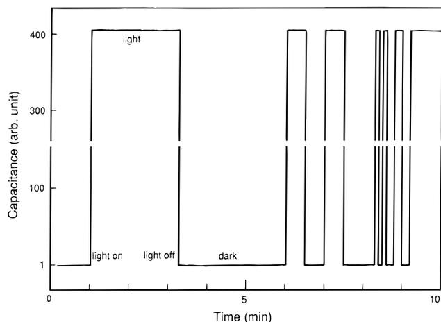
**FIGURE 13.** Response of the ITO/ZnOOEP/ $\text{SiO}_2/\text{Si}$  cell to irradiation as a function of time. A continuous sine-wave potential ( $-0.5$  to  $+0.5$  V) was applied. Reprinted with permission from ref 8. Copyright 1996 The Electrochemical Society.
