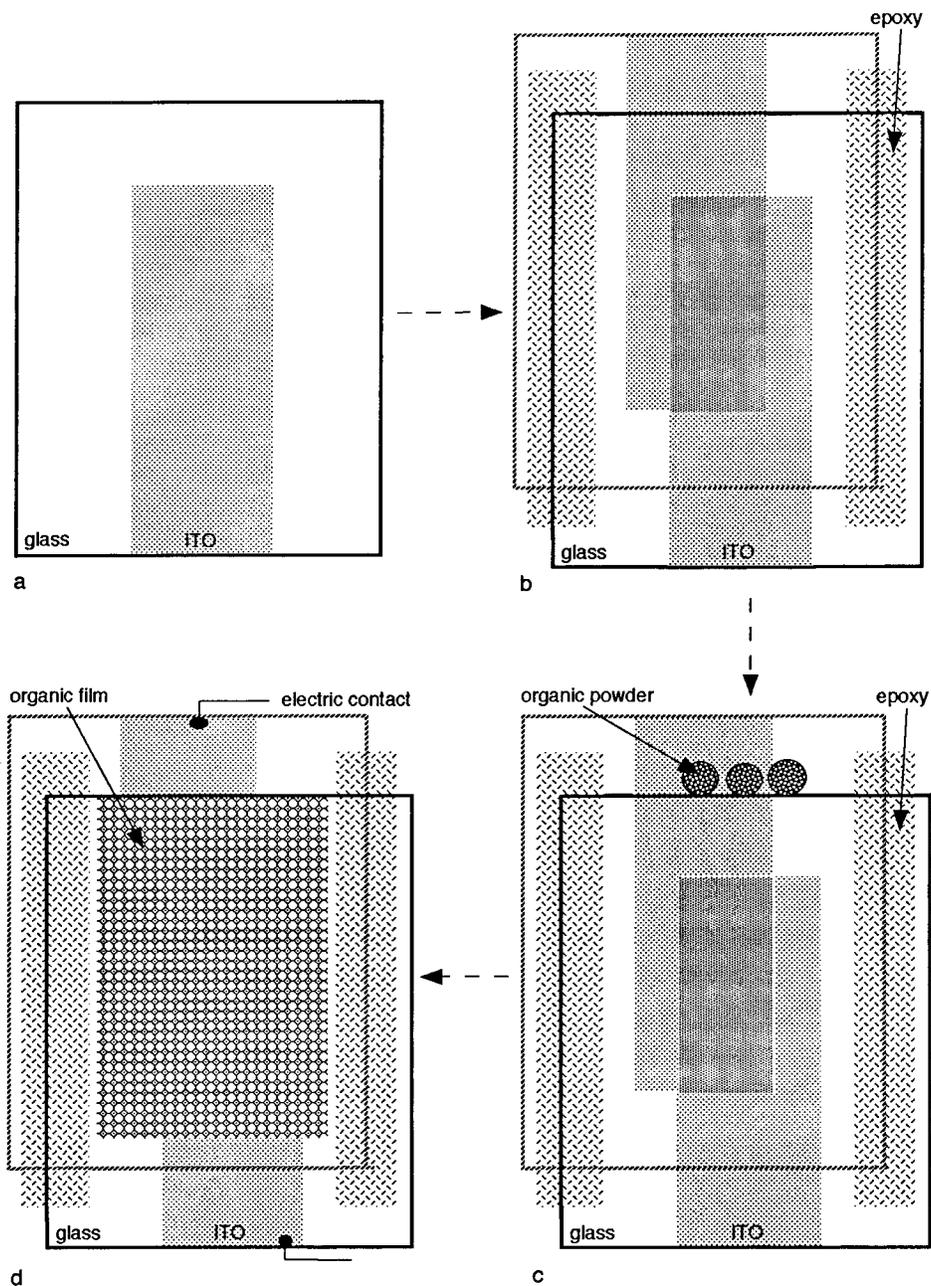
**FIGURE 1.** Schematic diagram of cell fabrication. (a) ITO removed on three sides. (b) Epoxy cement placed on the bare glass to adhere to another ITO (or metal) substrate and the substrates firmly pressed together to desired separation. (c) Organic powder placed at the opening and capillary-filled into the cell by heating to its melting point. (d) Cell cooled to room temperature and electrical contact to ITO made.
