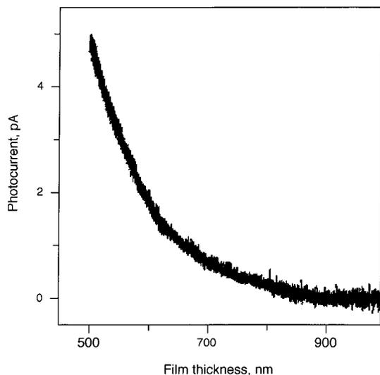
**FIGURE 14.** Relationship between the thickness of the Sudan I film and photocurrent under a bias of 5 V with tip positive. A sharp tip was moved through the layer (total film thickness  $\sim 1 \mu\text{m}$ ) at a rate of 5 nm/s. Reprinted from ref 10. Copyright 1998 American Chemical Society.
