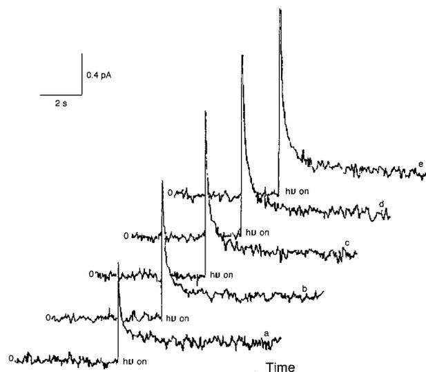
**FIGURE 17.** Photodischarge current as a function of time with Sudan I under short-circuit conditions. Charges were previously stored under potentials of (a) 2, (b) 4, (c) 6, (d) 8, and (e) 10 V. Reprinted from ref 10. Copyright 1998 American Chemical Society.
