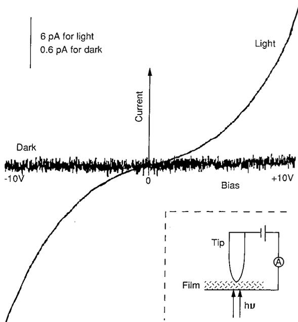
**FIGURE 15.** Current–voltage characteristics of a Sudan I thin film with a blunt tip contacting the film surface. Scan rate 0.2 V/s. The inset shows schematically the experimental setup. Reprinted from ref 10. Copyright 1998 American Chemical Society.
