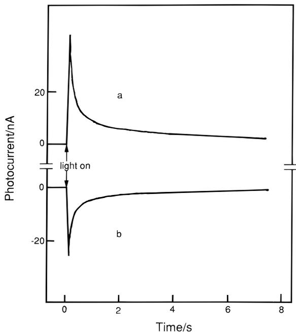
**FIGURE 8.** Short-circuit photocurrent of an ITO/ZnODEP/ITO cell as a function of time with a constant irradiation of 550 nm light after the cell had been subjected to irradiation with a 550 nm light beam under a bias of (a)  $-2$  and (b)  $+2$  V for 5 s followed by a rest period of 10 s under short-circuit conditions in the dark. Reprinted from ref 9. Copyright 1997 American Chemical Society.
