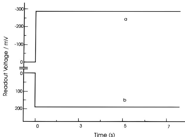
**FIGURE 10.** Readout voltage as a function of time. The data were stored by a single 10 ns laser pulse irradiation under potentials of (a)  $-1.0$  and (b)  $+1.0$  V. Reprinted from ref 9. Copyright 1997 American Chemical Society.
