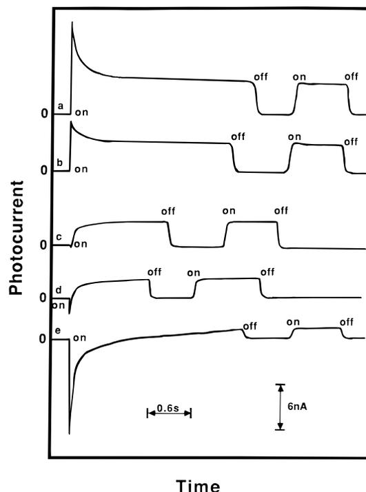
**FIGURE 9.** Photocurrent of an ITO/ZnODEP/ITO cell as a function of irradiation (550 nm) time under short-circuit conditions after irradiation of the cell with a 550 nm light under a bias of (a)  $-0.2$ , (b)  $-0.05$ , (c)  $+0.2$ , (d)  $+0.4$ , and (e)  $+1.2$  V for 5 s and a rest period of 10 s in the dark under short-circuit conditions. On and off indicate the irradiation is turned on and off. Reprinted from ref 9. Copyright 1997 American Chemical Society.
