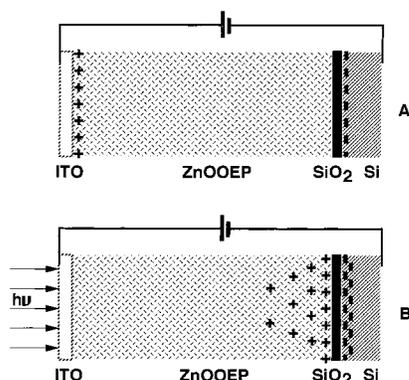
**FIGURE 11.** Schematic diagram of the operational principles for charge storage in a photoconductive medium (A) in the dark and (B) with irradiation. Reprinted with permission from ref 8. Copyright 1996 The Electrochemical Society.
