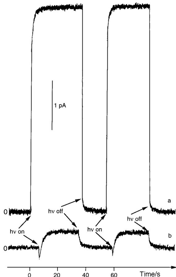
**FIGURE 6.** Short-circuit photocurrent, as a function of time, generated in crystal domains that were (a) purple and (b) blue in color. Of 16 separate domains sampled, the 5 smallest photocurrents were generated from green-blue- or blue-colored domains. The  $I_{sc}$  vs  $t$  curves for these 5 domains had the same shape as curve b while the other 11 domains generated curves similar to curve a. Reprinted from ref 14. Copyright 1997 American Chemical Society.
