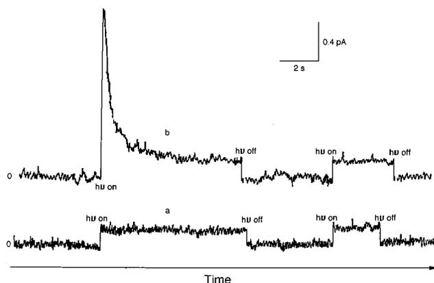
**FIGURE 16.** Short-circuit photocurrent as a function of time for Sudan I thin films where the sample (a) was not charged previously and (b) was previously photocharged under a bias of  $-10 \text{ V}$ . Reprinted from ref 10. Copyright 1998 American Chemical Society.
