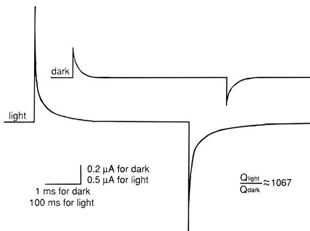
**FIGURE 12.** Charge and discharge characteristics of the cell with and without irradiation. A continuous square-wave potential ( $-0.4$  to  $+0.4$  V) was applied. Reprinted with permission from ref 8. Copyright 1996 The Electrochemical Society.
