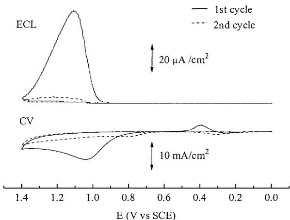
Figure 3. Cyclic voltammograms and ECL curves at  $\text{CH}_3(\text{CH}_2)_5\text{-SH}$  monolayer coated Au electrode in 0.15 M phosphate buffer solution (pH 7.5) containing 100 mM TPrA and 1  $\mu\text{M}$   $\text{Ru}(\text{bpy})_3^{2+}$ . Potential scan rate, 0.1 V/s.
