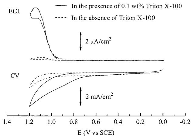
Figure 4. Cyclic voltammograms and ECL curves at a Pt electrode in 0.15 M phosphate buffer solution (pH 7.5) containing 100 mM TPrA and  $1 \mu\text{M}$   $\text{Ru}(\text{bpy})_3^{2+}$  in the presence and absence of 0.1 wt % Triton X-100. Potential scan rate, 0.1 V/s.
