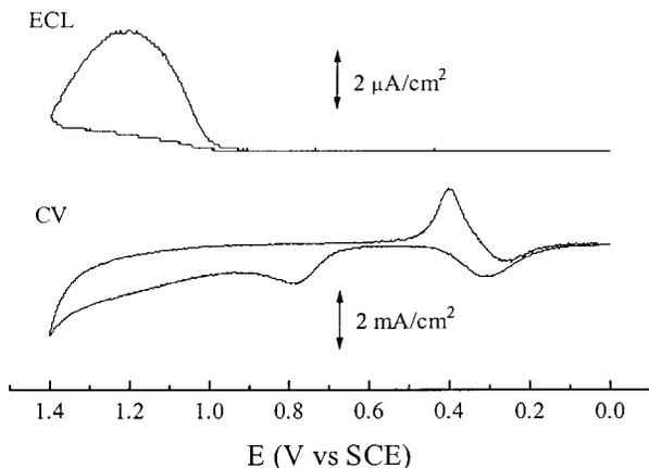
Figure 1. Cyclic voltammogram and ECL curve at a Au electrode in 0.15 M phosphate buffer solution (pH 7.5) containing 100 mM TPrA and 1  $\mu\text{M}$   $\text{Ru}(\text{bpy})_3^{2+}$ . Potential scan rate, 0.1 V/s.
