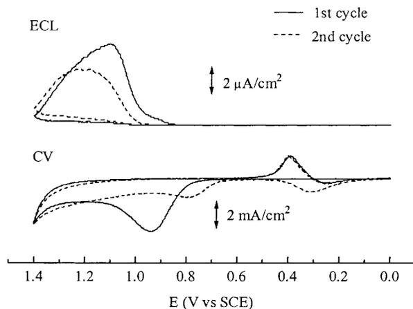
Figure 2. Cyclic voltammograms and ECL curves at a  $\text{HO}(\text{CH}_2)_6\text{SH}$ -monolayer-coated Au electrode in 0.15 M phosphate buffer solution (pH 7.5) containing 100 mM TPrA and 1  $\mu\text{M}$   $\text{Ru}(\text{bpy})_3^{2+}$ . Potential scan rate, 0.1 V/s.
