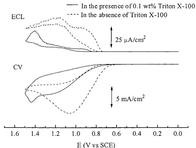
Figure 5. Cyclic voltammograms and ECL curves at a GC electrode in 0.15 M phosphate buffer solution (pH 7.5) containing 100 mM TPrA and  $1 \mu\text{M}$   $\text{Ru}(\text{bpy})_3^{2+}$  in the presence and absence of 0.1 wt % Triton X-100. Potential scan rate, 0.1 V/s.
