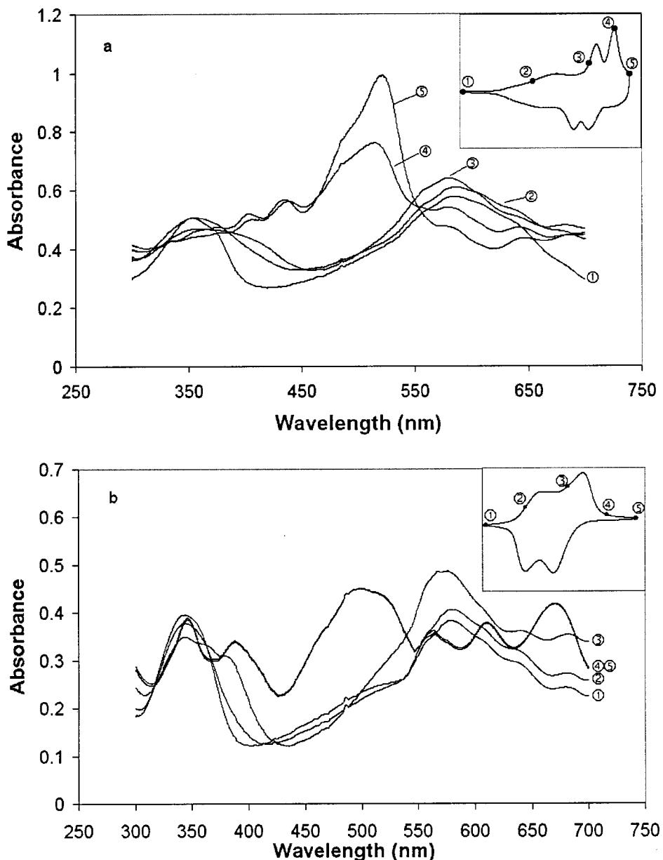
**Figure 4.** Absorption spectra at different potentials of (a) BBL and (b) BBB thin films on ITO in MeCN, 0.1 M TBAPF<sub>6</sub>. Insets show the potentials at which spectra were obtained.
