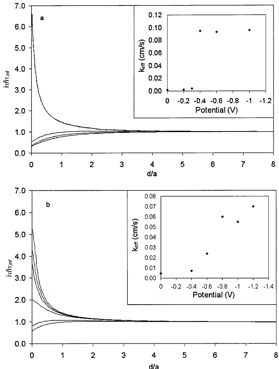
**Figure 6.** SECM tip ( $a = 12.5 \mu\text{m}$ ) approach curves with 5 mM TTF as redox mediator on (a) BBL and (b) BBB at different potentials. Potentials are from bottom to top: (a) 0.0, -0.2, -0.3, -0.4, -0.6, -0.8 V (last three curves are superimposed) and (b) 0.0, -0.4, -0.6, -0.8, -1.0, -1.2 V. Insets: Variation of  $k_{\text{eff}}$  with the potential applied to the film.
