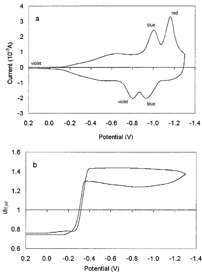
**Figure 2.** (a) Cyclic voltammetry of a BBL thin film spin-coated on an ITO electrode (surface area,  $1 \text{ mm}^2$ ) in MeCN, 0.1 M TBAPF<sub>6</sub>. The color of the film changed as indicated. (b) Tip current,  $i_T$ , recorded during the potential scan (scan rate, 20 mV/s). The tip was positioned by maintaining the film in the conductive state and recording an approach curve until  $i_T/i_{T,\infty} = 1.25$ .
