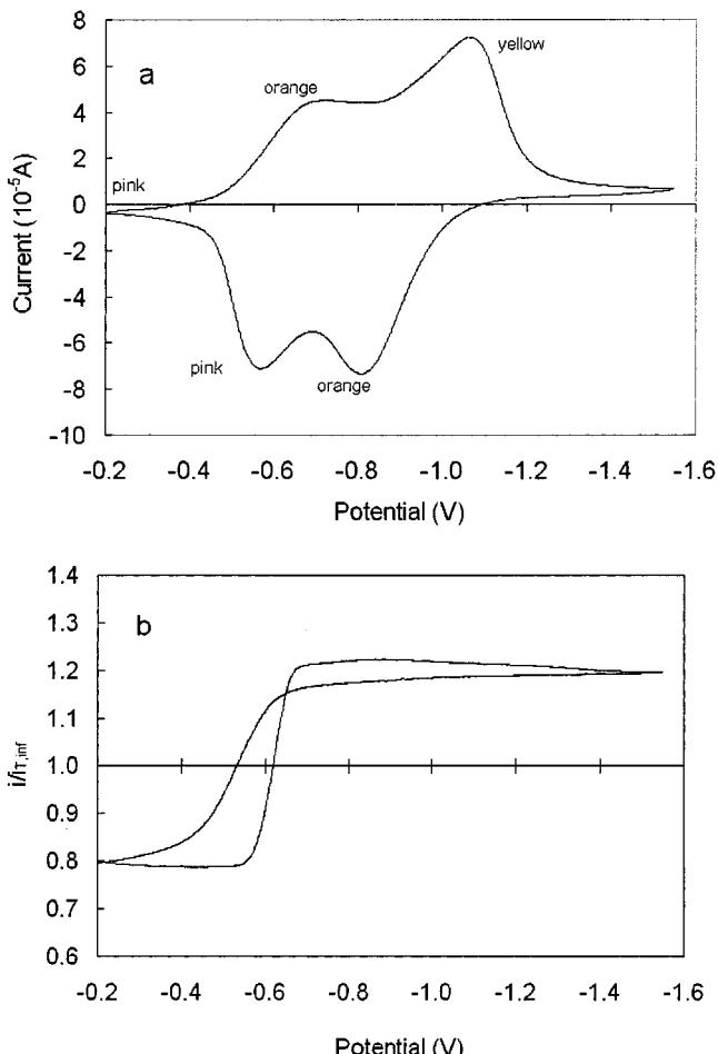
**Figure 3.** (a) Cyclic voltammetry of a BBB thin film spin-coated on an ITO electrode (surface area,  $3 \text{ mm}^2$ ) in MeCN, 0.1 M TBAPF<sub>6</sub>. The color of the film changed as indicated. (b) Tip current,  $i_T$ , recorded during the potential scan. Same experimental conditions as in Figure 2.
