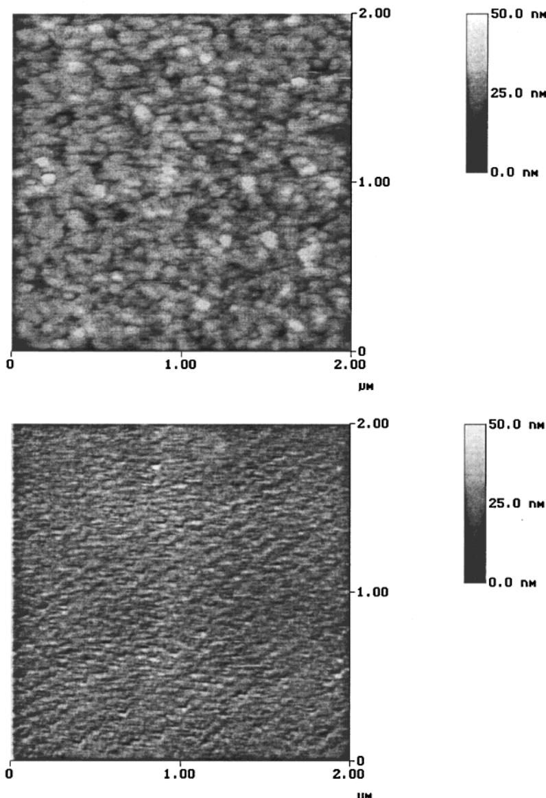
**Figure 5.** AFM images of (a) BBL and (b) BBB films deposited by spin-coating (2000 rpm, 30 s). The film thicknesses are (a) ~25 nm and (b) ~35 nm under these conditions (thicknesses obtained by AFM measurements).
