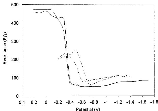
**Figure 8.** Resistance dependence of BBL (solid line) and BBB (dotted line) films during cyclic voltammetry. Experimental conditions as in Figure 2, except scan rate was 10 mV/s. The resistance was measured between the central microbands, whereas the potential was applied to the external microbands.
