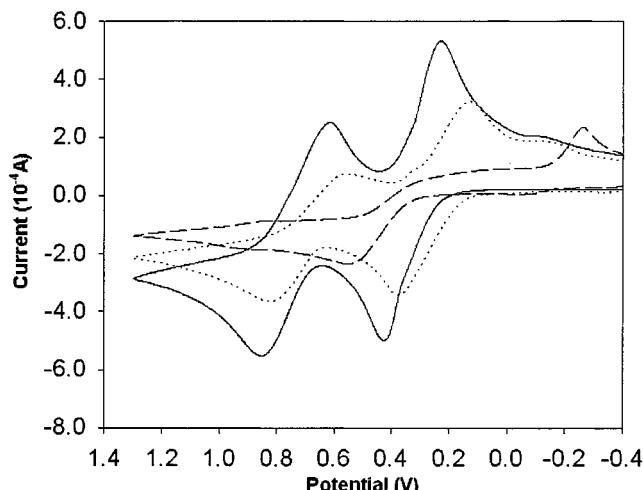
**Figure 7.** Cyclic voltammograms of 5 mM TTF in MeCN, 0.1 M TBAPF<sub>6</sub>, on a bare ITO electrode (solid line), BBL-coated ITO electrode (dotted line), and BBB-coated ITO electrode (dashed line).
