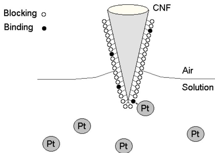
**Figure S3:** Schematic presentation of the nanoparticle collection technique showing a CFE tip modified with a surface layer containing a high ratio of nanoparticle blocking to binding molecules and positioned inside a colloidal Pt solution using SECM control.
