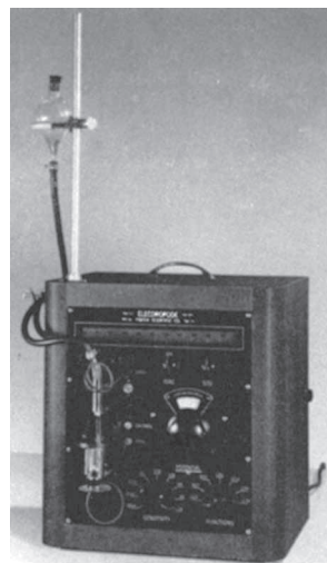
Figure 7. Manual polarographic instrument from Fisher Scientific Company, called the "Electropode".
