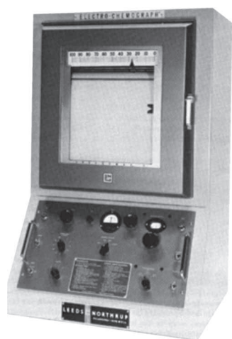
Figure 8. Polarographic instrument using a strip-chart recorder from Leeds & Northrup called the "Electrochemograph".
