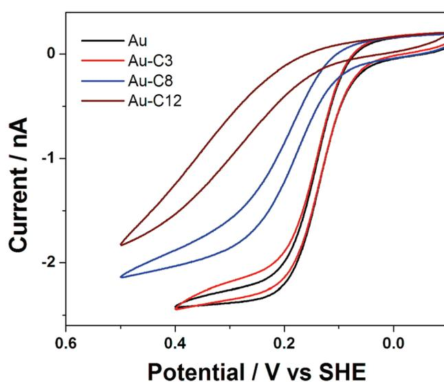
**Figure 4.** Cyclic voltammograms at Au UME in 1 mM ferrocenemethanol + 50 mM NaClO<sub>4</sub> before and after adding 10  $\mu\text{M}$  3-mercaptopropionic acid (C3), 8-mercaptooctanoic acid (C8), and 12-mercaptododecanoic acid (C12), respectively: scan rate 100 mV/s.
