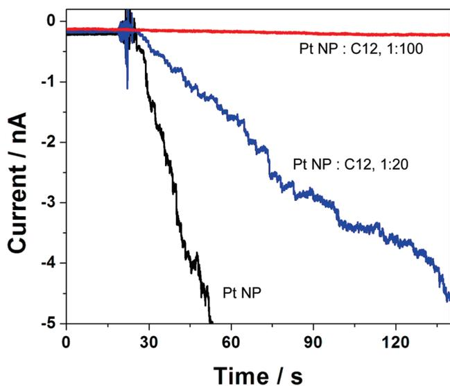
**Figure 7.** Current transients recorded at carbon UMEs before and after injection of Pt NPs capped by a mixture of citrate ions and C12 SAM. C UME  $8$   $\mu\text{m}$  in diameter, electrode potential  $0.45$  V, Pt NPs  $\sim 3.6$  nm, particle concentration  $50$  pM, electrolyte  $12$  mM hydrazine +  $50$  mM PBS buffer, pH  $\sim 7.5$ .
