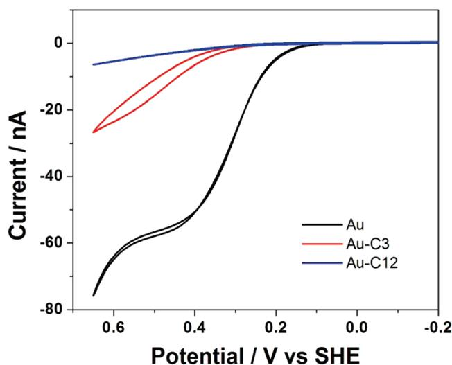
**Figure 2.** Cyclic voltammograms at Au UME in 12 mM hydrazine + 50 mM PBS before and after adding 10  $\mu\text{M}$  3-mercaptopropionic acid (C3) and 12-mercaptododecanoic acid (C12), respectively: scan rate 100 mV/s.
