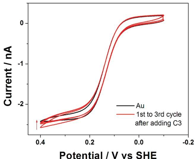
**Figure 3.** Cyclic voltammograms at Au UME in 1 mM ferrocenemethanol + 50 NaClO<sub>4</sub> before and after adding 50  $\mu\text{M}$  3-mercaptopropionic acid (C3): scan rate 100 mV/s.
