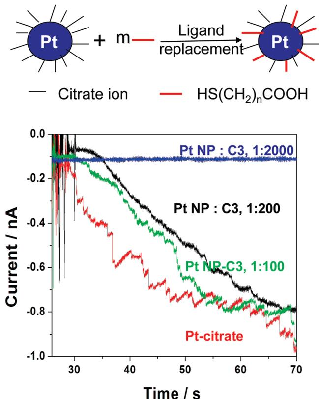
**Figure 6.** Current transients recorded at Au UMEs before and after injection of Pt nanoparticles capped by a mixture of citrate ions and C3 SAMs. Replacement of citrate by SAMs is illustrated at the top of the figure. Au UMEs  $10$   $\mu\text{m}$  in diameter, electrode potential  $0.1$  V, particle size  $\sim 3.6$  nm, particle concentration  $\sim 50$  pM, electrolyte  $12$  mM hydrazine +  $50$  mM PBS buffer, pH  $\sim 7.5$ .
