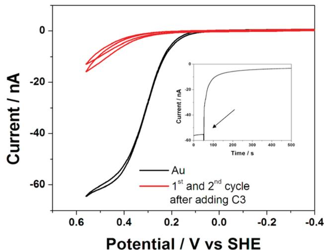
**Figure 1.** Cyclic voltammograms at Au UME in 12 mM hydrazine + 50 mM PBS before and after adding 50  $\mu\text{M}$  3-mercaptopropionic acid (C3): scan rate 100 mV/s. The inset figure shows the current transient before and after injection at 0.45 V.
