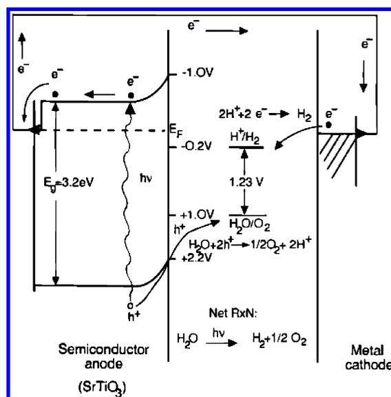
**Figure 8.** Typical semiconductor band diagram with respect to thermodynamic (multielectron transfer) half-reactions in solution for water splitting for SrTiO<sub>3</sub>/solution/Pt photoelectrochemical cell. Adapted with permission from Nozik, A. J.; Memming, R. J. *Phys. Chem.* **1996**, *100*, 13061. Copyright 1996 American Chemical Society.
