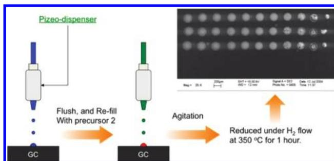
**Figure 5.** Method of array preparation using a dispenser. The piezo-dispenser is moved with a stepping motor under computer control and dispenses a designated number of drops of different solutions on substrate (e.g., glassy carbon); this is then subjected to an appropriate treatment (e.g., precipitation, reduction, oxidation) to produce the desired multicomponent array.
