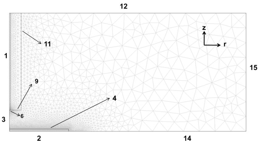
**Figure S4:** The mesh distribution of Comsol Multiphysics model in 2-D axial symmetry.
