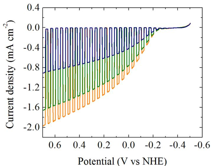
Figure S6. Linear sweep voltammogram of  $\text{W}/\text{Mo-BiVO}_4$  with chopped light under UV-Visible irradiation in 0.1 M  $\text{Na}_2\text{SO}_4$  and 0.1 M  $\text{Na}_2\text{SO}_4$  aqueous solution (pH 7). Beam intensity was gradually increased from 100 (blue), 300 (green) to 400  $\text{mW cm}^{-2}$  (yellow) with full output from a xenon lamp. Scan rate was 20  $\text{mV s}^{-1}$ .
