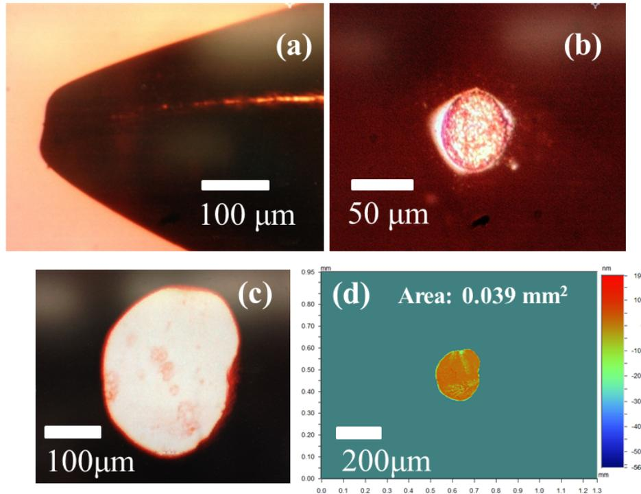
Figure S1. Optical microscopic images of Au UME from side (a) and top (b), and the image of the W/Mo-BiVO<sub>4</sub> photoanode covered by the insulating layer (c). Optical surface profiler images of the photoanode (d) that is identical W/Mo-BiVO<sub>4</sub> shown in (c). The optical profiler was used to measure the exposed area of the photoanode (0.039 mm<sup>2</sup>) and to measure the thickness of the insulating Teflon layer on the photoanode (~ 20 μm).
