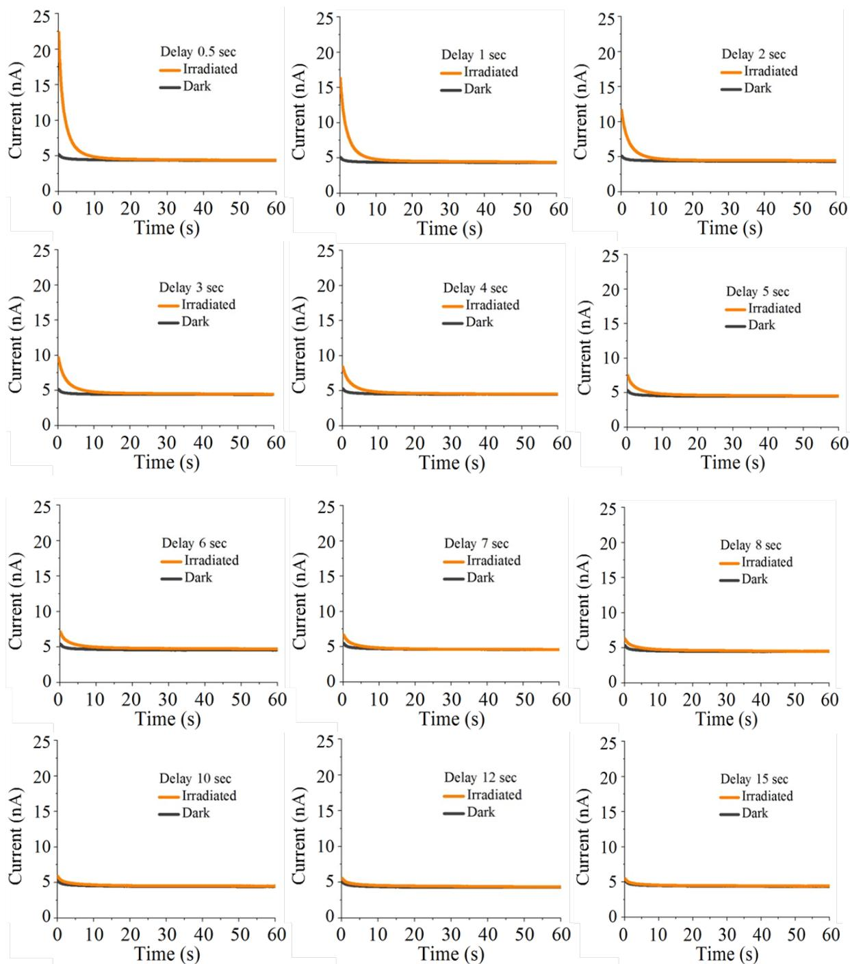
Figure S4. Chronoamperograms (CAs) of surface interrogation using Au UME on the W/Mo-BiVO<sub>4</sub> electrode with different decay times from 0.5 s to 15 s after UV-Visible irradiation for 5 s (yellow). CA of that without the irradiation is shown as a grey solid line. The potential of Au
