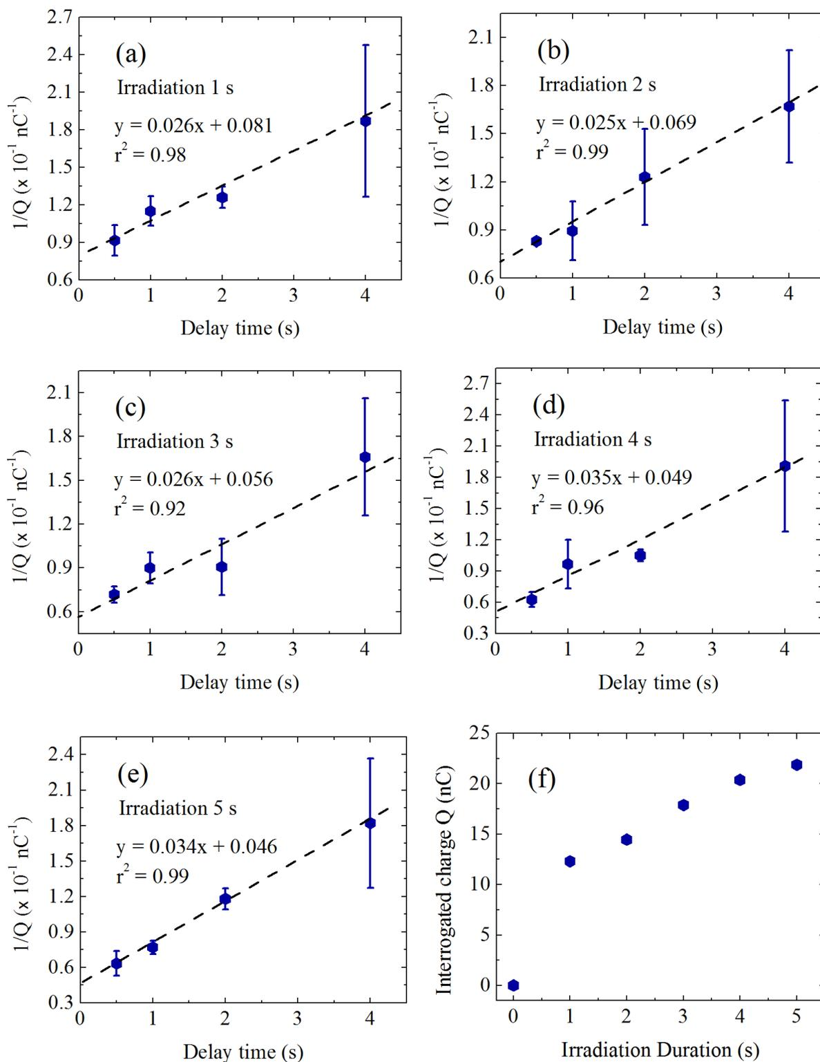
Figure S5. Interrogated charges of OH• at W/Mo-BiVO<sub>4</sub> with various irradiation durations of (a) 1, (b) 2, (c) 3, (d) 4, and (e) 5 s. For each measurement, four different decay times were allowed
