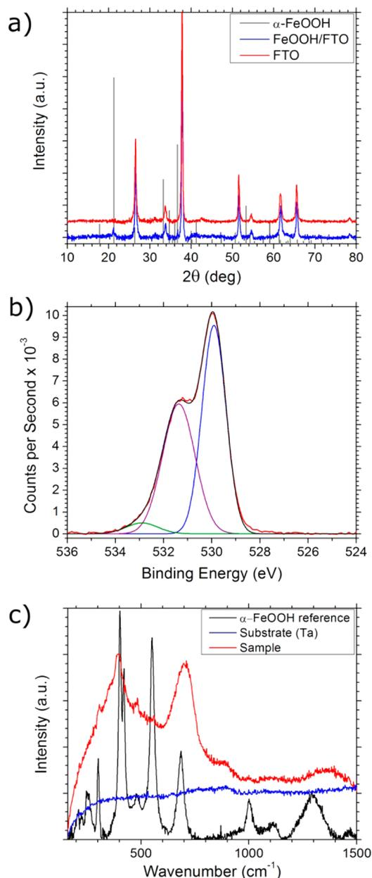
**Figure 3.** (a) XRD patterns for FTO substrate (red) and  $\sim 5 \mu\text{m}$  thick FeOOH deposited on FTO (blue). The one peak not attributable to FTO matches  $\alpha$ -FeOOH. (b) XPS spectrum for O(1s) region of FeOOH. (c) Raman spectra of FeOOH films on Ta foil. Good agreement is seen between  $\alpha$ -FeOOH peak positions; however, the peaks are significantly broader and very weak.
