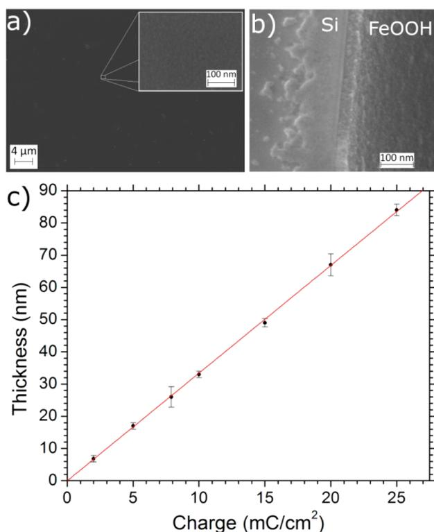
**Figure 1.** (a) SEM image of FeOOH on Si wafer, showing smoothness and uniformity over a large area. (b) Cross-sectional ( $75^\circ$ ) SEM of FeOOH on Si wafer, giving a better view of the surface roughness compared to the film thickness. (c) Thickness as determined by ellipsometry versus charge passed during deposition, showing high linearity with a relationship of  $3.3 \text{ nm}/\text{mC}/\text{cm}^2$ .
