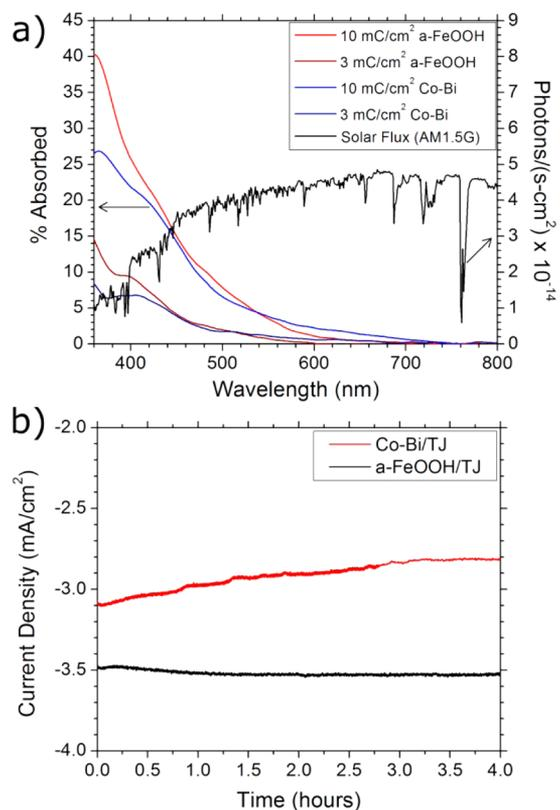
**Figure 6.** (a) Absorption spectra of a-FeOOH and Co-B<sub>i</sub> films on FTO measured using an integrating sphere (left axis) and AM1.5G spectra converted to photon flux (right axis). (b) Stability tests of a-FeOOH/TJ and Co-B<sub>i</sub>/TJ devices in 1 M Na<sub>2</sub>CO<sub>3</sub> at 0 V vs RHE measured in a three-electrode configuration, each trace is the average of four different tests, so a total of eight devices are represented in this plot.
