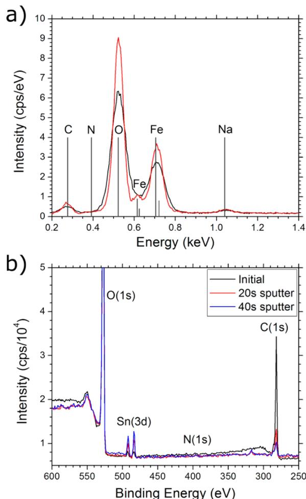
**Figure 2.** (a) EDS spectra of  $\sim 350$  nm thick FeOOH on FTO substrate. (b) XPS spectra of  $\sim 30$  nm thick FeOOH before and after  $\text{Ar}^+$  sputtering. Both figures show no evidence of N anywhere in the films.
