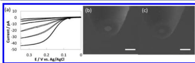
**Figure 2.** (a) CVs in 1 mM FcMeOH, 0.2 M NaCl after each  $\text{TiO}_2$  deposition step. (b,c) SEM images of bare Pt UME milled by FIB (b) and  $\text{TiO}_2$  deposited Pt UME (c). Scale bars = 500 nm.
