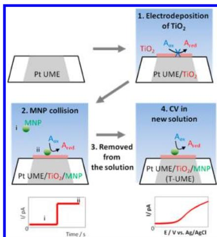
**Figure 1.** Schematics of the fabrication and the characterization of T-UME by electrodeposition of  $\text{TiO}_2$  on Pt UME, collision with MNP, removal of UME from the solution, and running CV in new solution without additional MNPs.
