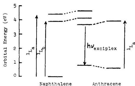
Figure 3. Schematic representation of the stabilization of the excited anthracene-naphthalene sandwich pair. The orbital energies are derived from photoelectron spectroscopic energies<sup>6,7</sup> and optical absorption spectra. The zero has been set at the highest bonding level of naphthalene and the mixed excimer fluorescence is indicated schematically.
