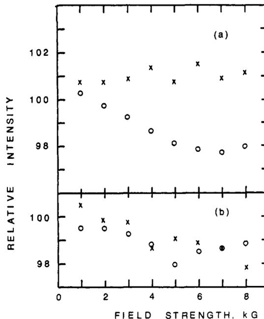
Figure 2. (a) Magnetic field effect on delayed fluorescence (emission at 390 nm) from a  $2.6 \times 10^{-4} M$  solution of pyrene in DMF: O, no oxygen,  $\tau = 1.4$  msec; ×, added oxygen,  $6 \times 10^{-3}$  atm,  $\tau = 0.7$  msec. (b)  $2.0 \times 10^{-4} M$  pyrene in acetonitrile: O, no oxygen,  $\tau = 2.1$  msec; ×, added oxygen,  $2.2 \times 10^{-5}$  atm,  $\tau = 1.4$  msec.
