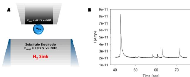
**Figure 4.** (A) Schematic representation of the use of the SECM in tip generation–substrate collection mode. The C fiber UME was poised at  $-0.3 \text{ V vs NHE}$  to drive the proton reduction reaction on the Pt nuclei that would form, and the substrate electrode was poised at  $0.2 \text{ V vs NHE}$  to oxidize the hydrogen gas to protons. (B) Representative data collected during the SECM experiment with  $100 \text{ fM PtCl}_6^{2-}$ .
