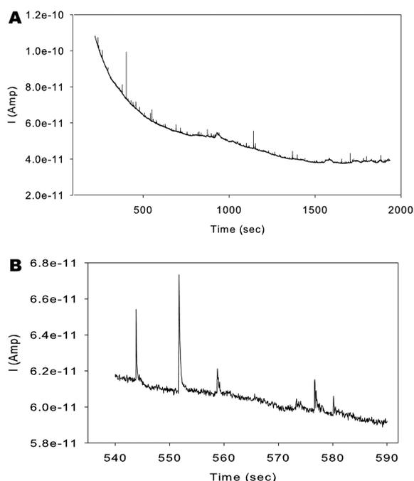
**Figure 2.** (A) Typical amperometric  $i-t$  response on a 10  $\mu\text{m}$  C fiber UME in 1 M sulfuric acid solution, where the concentration of hexachloroplatinate was 60  $\mu\text{M}$ . The applied potential was  $-0.15$  V vs NHE. (B) Enlargement of some of the data indicating the typical shape of the blips in the presence of hexachloroplatinate.
