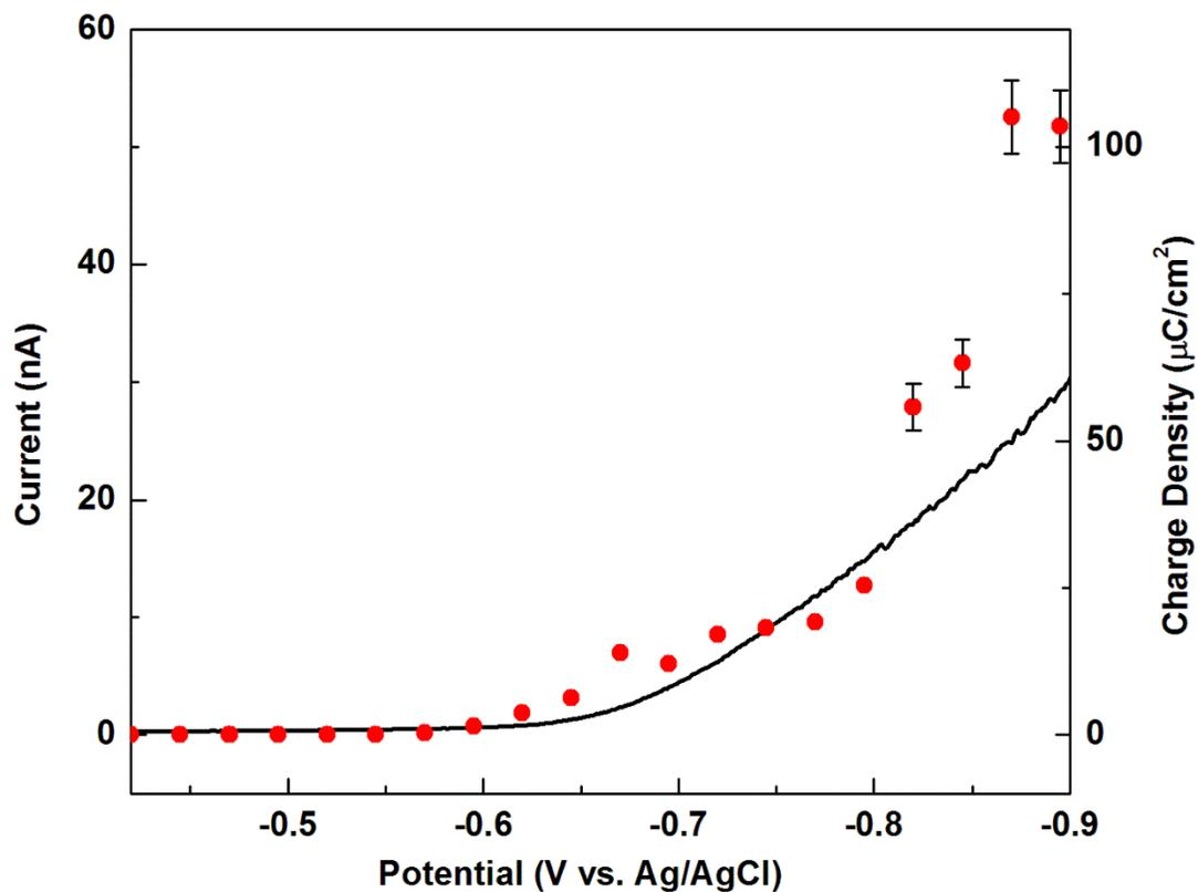
**Figure S6.** Zoomed in view of the MoS<sub>2</sub> surface redox titration curve. A reduction event observed in potentials -0.62 V to -0.8 V is attributed to the reduction of residual MoS<sub>3</sub> in the film.<sup>2</sup> Similar reduction event in the bulk of the film is also observed in the LSV shown in Figure S4.
