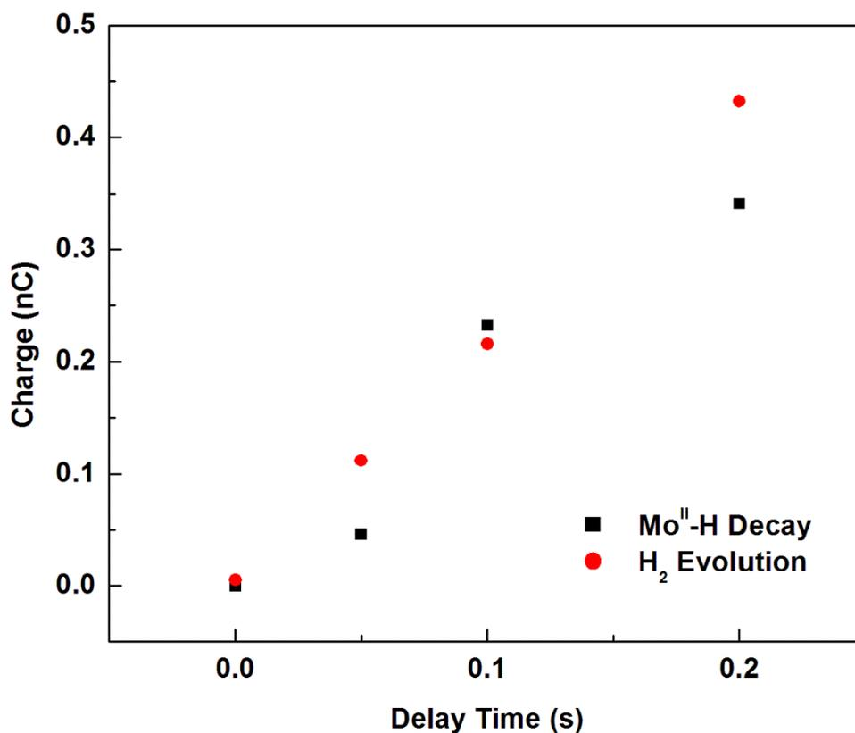
**Figure S8.** A plot of Mo-H decay and H<sub>2</sub> evolution as a function of  $t_{\text{delay}}$  (in pH 5.3, at 600 mV overpotential).
