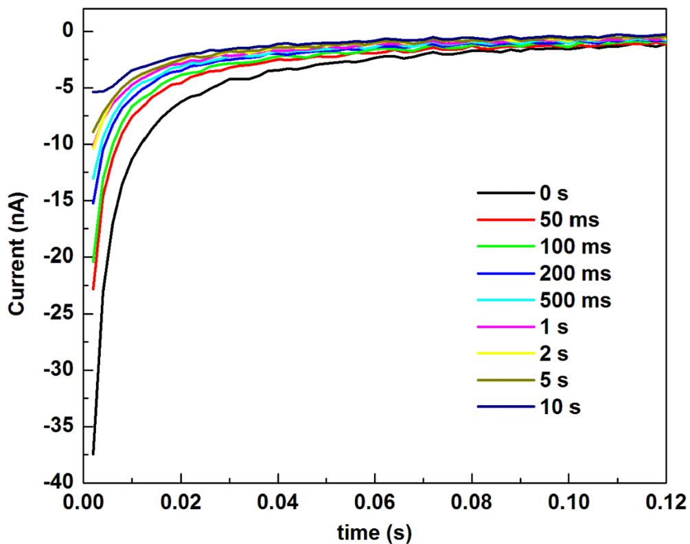
**Figure S7.** Titration chronoamperograms at -1.12 V with varying  $t_{\text{delay}}$ . A systematic decrease in the titration currents correspond to consumption of the active species Mo-H by the solvated protons via HER during the delay time. The integrated charge densities from this plot are plotted in Figure 3.
