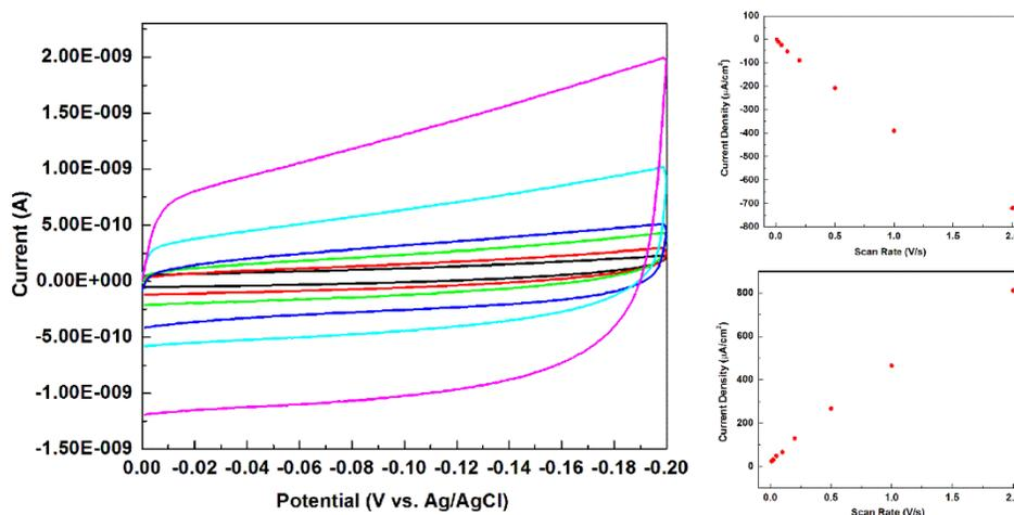
**Figure S5.** Cyclic voltammograms of non-Faradaic charging of the MoS<sub>2</sub> electrodes at varying scan rates from 10 mV/s to 2 V/s. Charging currents (two figures on the right) were plotted as a function of scan rate (for both forward and backward scans) to yield the double layer capacitance as the slope.
