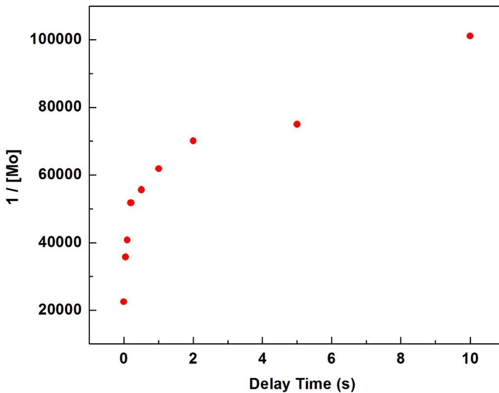
**Figure S10.** A plot of  $1/[Mo]$  vs.  $t_{\text{delay}}$  at substrate potential  $-1.12$  V. Non-linearity across all time ranges indicate that the reaction is not second order in Mo-H.
