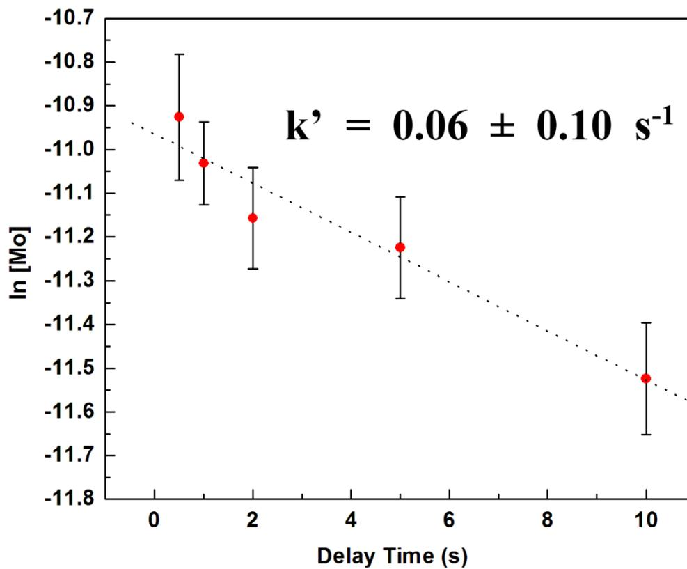
**Figure S9.** A plot of  $\ln [\text{Mo}]$  vs.  $t_{\text{delay}}$  for  $t_{\text{delay}} > 200 \text{ ms}$  (at substrate potential  $-1.12 \text{ V}$ ). A rate constant similar to that obtained at  $-0.92 \text{ V}$  (14 % hydride coverage) was observed.
