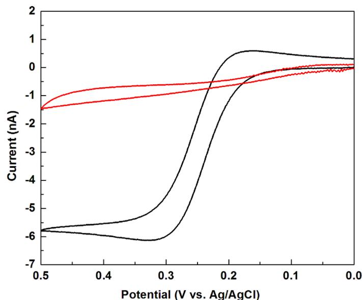
**Figure S3.** Cyclic voltammograms arising from the oxidation of 1.8 mM FcDM to FcDM<sup>+</sup> in pH 7 phosphate buffered water (Scan rate 50 mV/s). Black trace is that of a clean 25 μm Au UME, and red trace is that of a MoS<sub>2</sub> deposited 25 μm Au UME. MoS<sub>2</sub> deposition covered the underlying Au UME completely, evidenced by the negligible Faradaic current in the deposited electrode.
